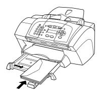
Adjust the left paper guide against the envelopes (be careful not to bend the envelopes). Make sure the envelopes fit within the tray (do not overload it).
