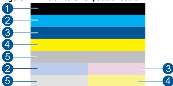
Figure 11-1 Color bars - expected result
