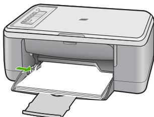
7. Make sure the print settings, paper size and type, match the paper loaded in the input tray.
