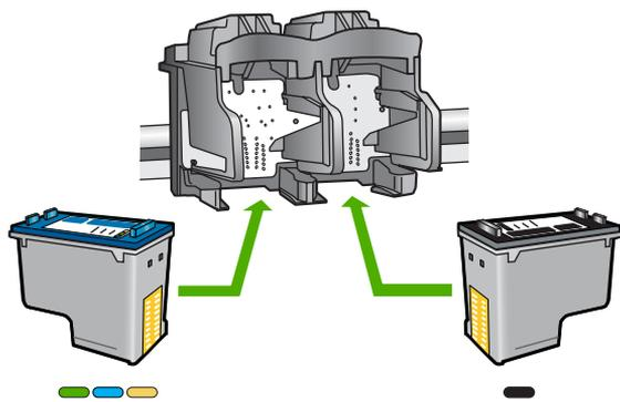
**To make sure the print cartridges are installed correctly**
