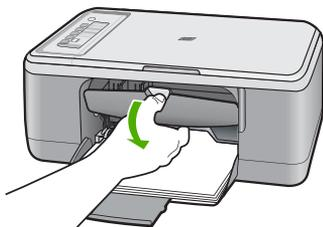
3. Make note of where the print carriage is stuck and look for jammed paper. A paper jam can cause the error message and the print carriage to stall.
