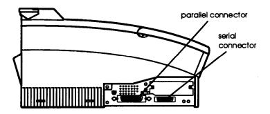
Parallel cables should be the twisted-pair shielded type.
