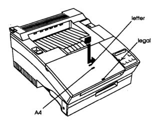
6. Make sure the paper path selector on the top left corner of the printer is set to the face-down position.
