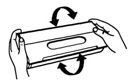
Insert the imaging cartridge into the printer by placing the pins on each side of the cartridge into the grooves inside the printer. Slide it gently into the opening until it stops.
