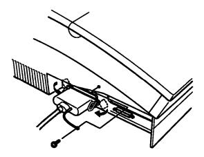
For the serial connector, use a screwdriver to fasten the screws of the connector, if required. If your cable has a grounding wire, connect it to the printer's ground connector as shown.
