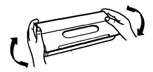
5. Set the imaging cartridge on a clean, flat surface. Firmly grip the tab on the left side of the imaging cartridge. Pull the clear seal all the way out with firm, even pressure as shown.
