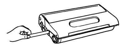
Hold the imaging cartridge and gently shake it from front to back.
