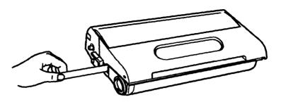
4. Hold the imaging cartridge and gently shake it from front to back.
