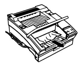
2. If the paper tears when you remove it, make sure you remove any pieces remaining in the printer. To do this, gently open the printer cover.
