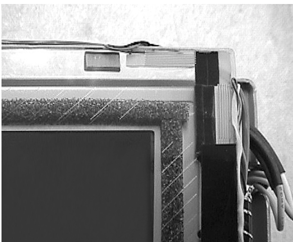
Figure 2.9 Attaching double-sided adhesive tape to the touchscreen
