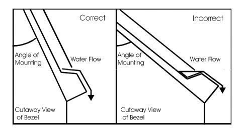
Figure 1-3. Mounting to Prevent Moisture Accumulation
