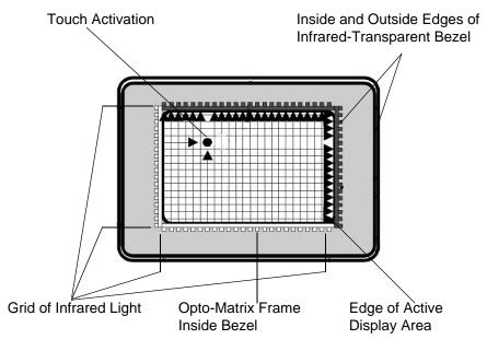
Figure 1-1. Scanning Infrared Technology
