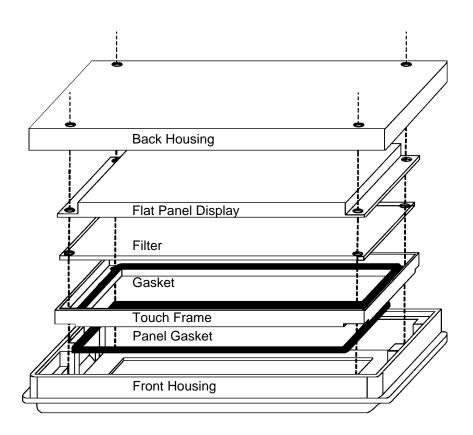
Figure 2-6. Industrial or Medical Mounting Method
