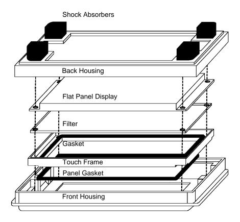
Figure 2-5. Anti-Shock/Vibration Mounting Method
