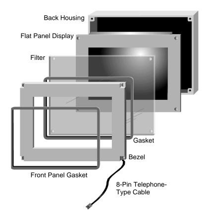
Figure 2-3. Typical NEMA 4 Mounting Method (Front View)
