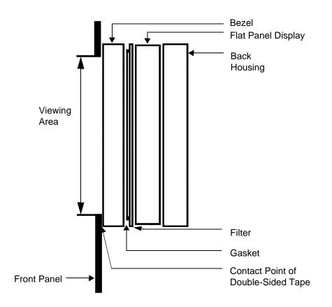
Figure 2-2. Simplest Mounting Method (Side View)
