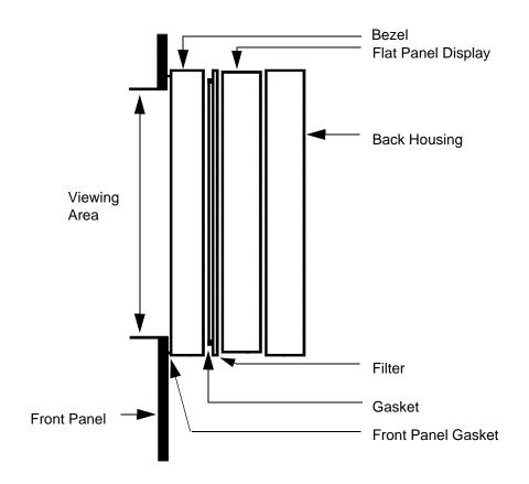
Figure 2-4. Typical NEMA 4 Mounting Method (Side View)
