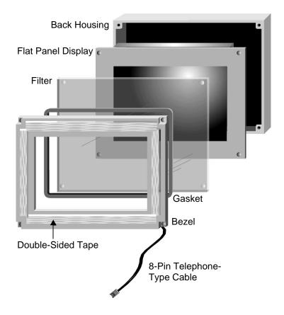
Figure 2-1. Simplest Mounting Method (Front View)
