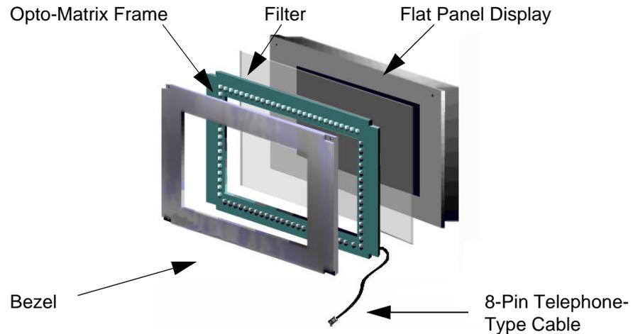
Figure 1-2. Modular Flat Panel Touch System Components
