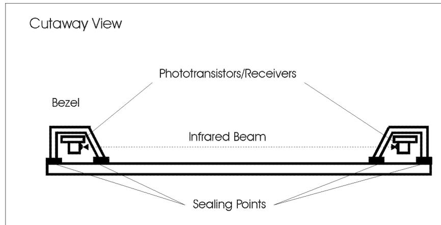
Figure 4-1. Modular Flat Panel Touch System Sealing
