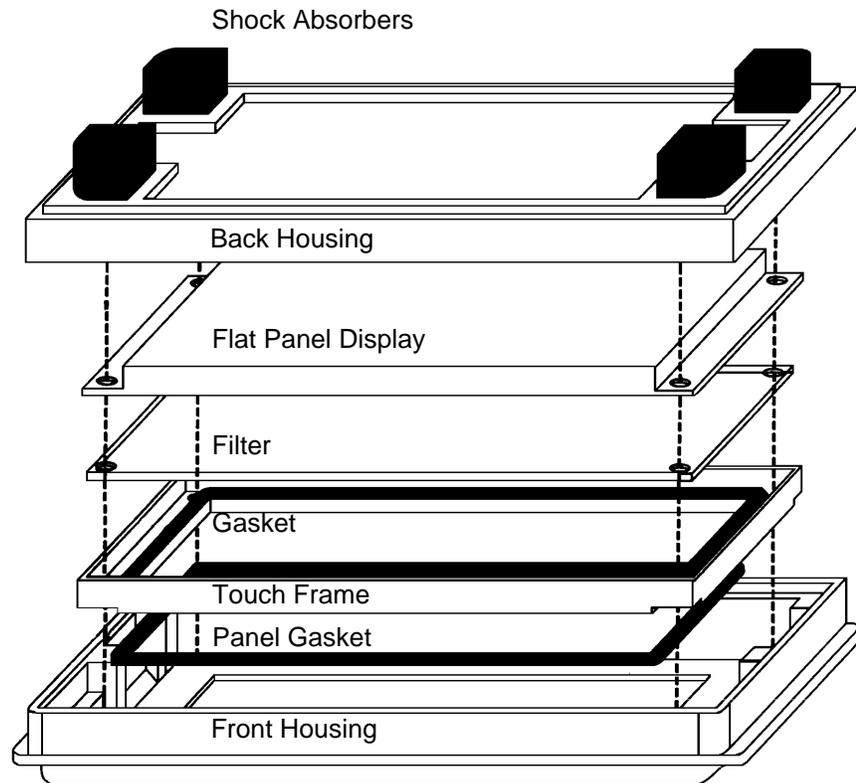
Figure 2-5. Anti-Shock/Vibration Mounting Method
