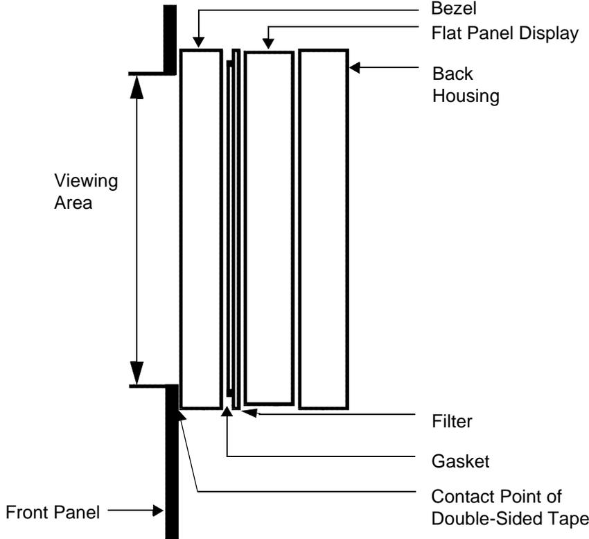
Figure 2-2. Simplest Mounting Method (Side View)
