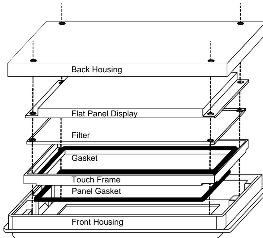
Figure 2-6. Industrial or Medical Mounting Method
