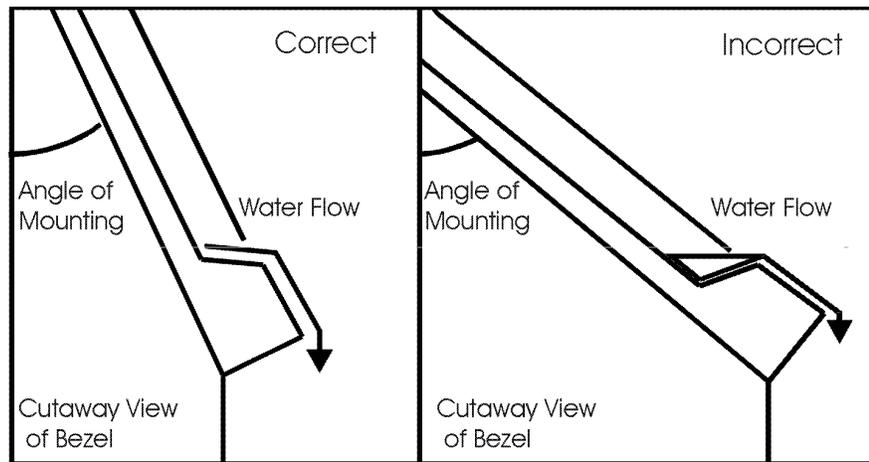
Figure 1-3. Mounting to Prevent Moisture Accumulation
