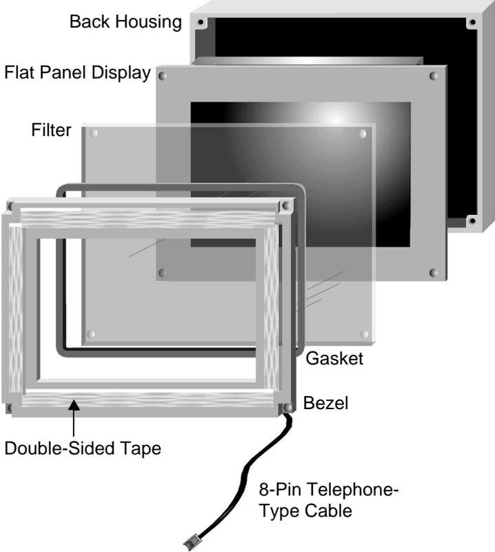
Figure 2-1. Simplest Mounting Method (Front View)
