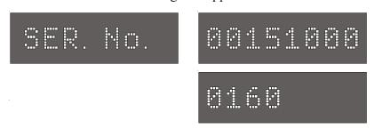
The most significant eight digits of the serial number are displayed first, after pressing the Set button the last four digits are shown.
