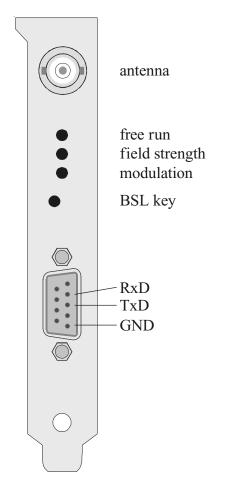
The rear panel includes the antenna connector, three status LEDs, the BSL button, and a 9 pin sub D connector (see figure below).
