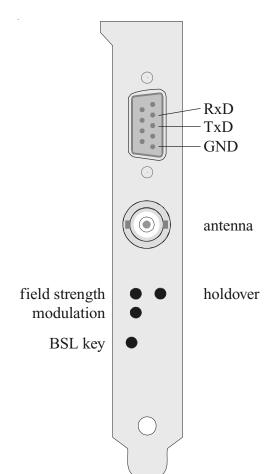
The rear panel includes the antenna connector, three status LEDs, the BSL button, and a 9 pin sub D connector (see figure below).
