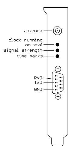
change when the minute changes (seconds increment from 59 to 0). The brightness of the LED in the middle depends on the strength of the RF signal. The lower, green LED should be blinking exactly once per second corresponding to the time marks from DCF77. If this LED flashes there is some electrical noise around which prevents the receiver from decoding the time marks and synchronizing. All information given by these LEDs can also be obtained from the screen of the program PCPSINFO.EXE.
