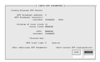
The NTP configuration page is used to set up the additional NTP parameters needed for a more specific configuration of the NTP subsystem.
