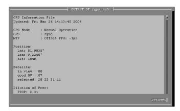
Using the button "List detailed GPS information" gives you the possibility to check detailed GPS status information. The first parameter indicates the time and date of the last update of the shown parameters. Next you find the GPS receiver status and the NTP status, followed by the GPS position data. The position uses the Latitude / Longitude / Altitude format. Latitude and Longitude are shown in degrees, minutes and seconds, Altitude is shown in meters above WGS84 ellipsoid.
