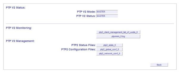
By selecting the **ptpmmm\_0.log** button more than 100 PTP nodes can be listed. The list of PTP nodes with their current status information has the following form:
