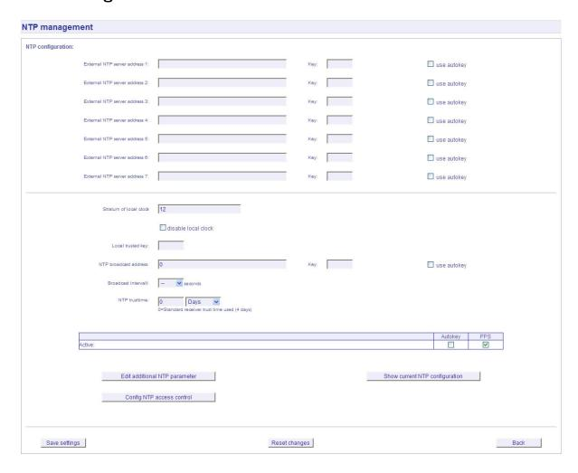
The NTP configuration page is used to set up the additional NTP parameters needed for a more specific configuration of the NTP subsystem.
