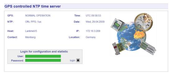
On this start page you see a short status display, which corresponds with the LC display on the front panel of the LANTIME unit. The upper line shows the operation mode of the receiver.
