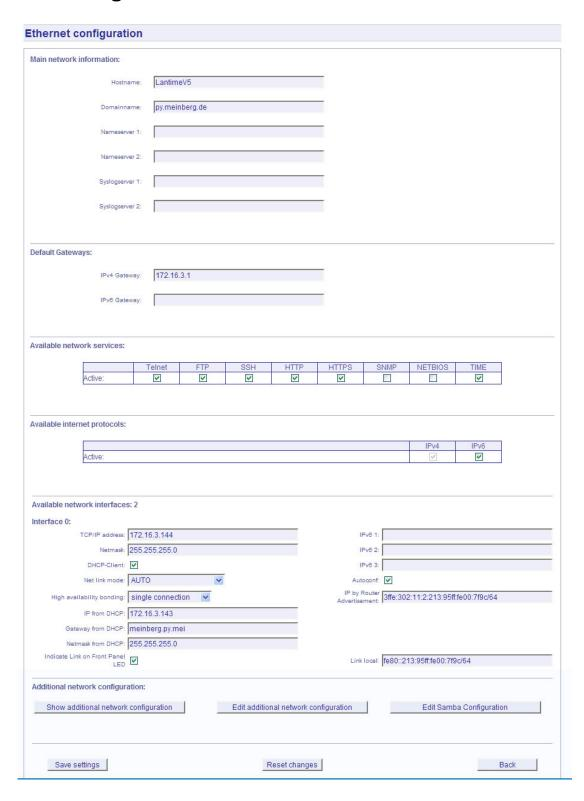
In the network configuration all parameters related to the network interfaces can be changed. In the first section you can change the hostname and domain name. You can also specify two nameserver and two SYSLOG server. In the nameserver and syslog server fields you may enter an IPv4 or IPv6 address (the syslog servers can be specified as a hostname, too).
