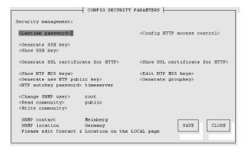
The password is stored encrypted on the internal flash disk and can only be reset to the default value "timeserver" by a "factory reset", changing all settings back to the factory defaults. Please refer to the LCD configuration
