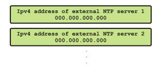
Seven additional external NTP servers can be set up to provide a high grade of redundancy for the internal reference clock.
