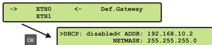
There is a separate configuration submenu for every physical network interface. If there is no DHCP client mode activated a static IP address for each interface can be entered. IPv4 addresses are built of 32 bits which are grouped in four octets, each containing 8 bits. You can specify an IP address in this mask by entering four decimal numbers, separated by a point ".".
