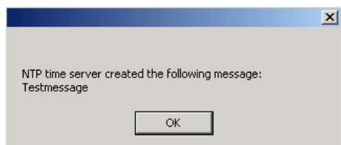
You can send messages via the special Windows protocol in your local network. It is not necessary to enable the NETBIOS protocol of the LANTIME in order to use this notification. On the Windows client side it is necessary to activate the "Microsoft Client for Windows" in the network configuration.
