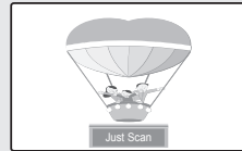
Just Scan Use this function to see the full image without cutting off the picture when DTV or HDMI 1080i/1080p signals are input.
