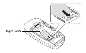
Note: If the card is not inserted correctly, the phone will not detect the SIM card. Remove the battery and re-orient the card back into the slot.
