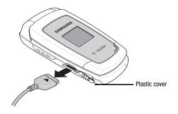
Note: Failure to unplug the travel adapter before you remove the battery, can cause the phone to become damaged.
