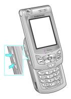
In Idle mode with the slider pushed up, you can also adjust the keypad tone volume using these keys.
