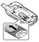
**4.** Place the battery so that the tabs on the end align with the slots at the bottom of the phone.
