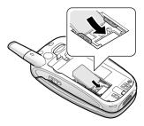
To remove the SIM card, slide it upwards, as shown, and take it out of the socket.
