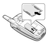
**5.** Replace the battery so that the tabs on the end align with the slots at the bottom of the phone.
