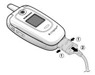
**Note:** You must unplug the charger before removing the battery from the phone during charging, otherwise, the phone could be damaged.
