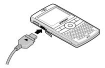
**Note:** The following illustration shows the **correct** and **incorrect** method for connecting the charger. Verify the arrow on the adapter is showing and pointing to the handset for a correct connection. If it is not, damage to the accessory port will occur therefore voiding the phones warranty.
