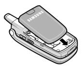
2. Press the battery down until it clicks into place. Make sure that the battery is properly installed before switching on the phone.
